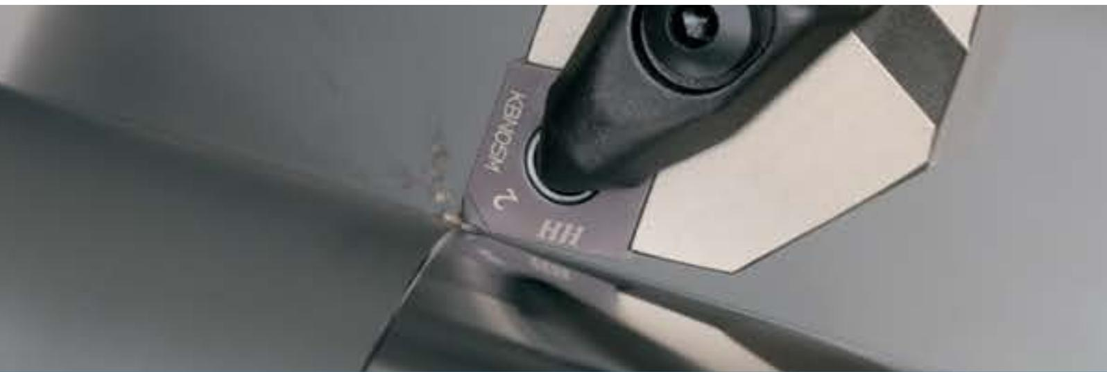
Excellent chip control when machining hardened material
