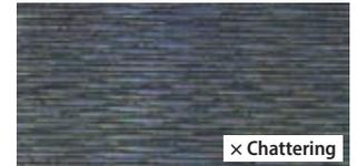
Cutting conditions:  $V_c = 80$  m/min,  $a_p = 12$  mm,  $f = 0.03$  mm/rev, wet (Oil-based)
