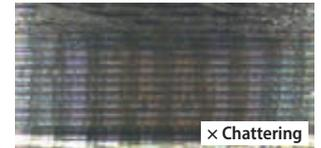
Cutting conditions:  $V_c = 80$  m/min,  $a_p = 8$  mm,  $f = 0.05$  mm/rev, wet (Oil-based)
