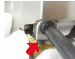
4. Loosen the cartridge clamp screw (Fig. 4).
