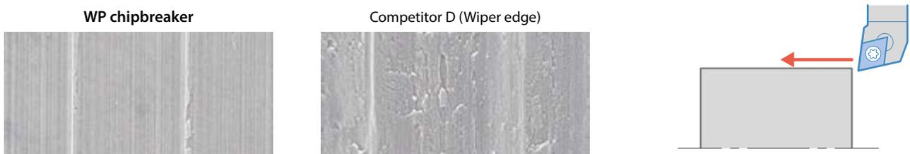
Cutting conditions:  $V_c = 80$  m/min,  $a_p = 0.73$  mm,  $f = 0.05$  mm/rev, wet Insert: CCMT09T304 type Workpiece: ST45 (steel pipe)
