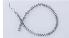
WP chipbreaker improved chip control compared to competitor G. Machining efficiency was improved by increasing feed rate. Tool life extended to 1.5 times that of Competitor G.
