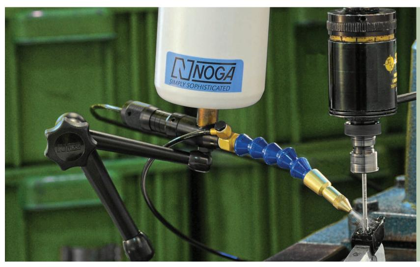
**COBRA** 's drop ejector is designed to accurately shoot small quantities of liquid to distinct targets. An air actuated piston shoots the drops through a flexible hose onto the target.
